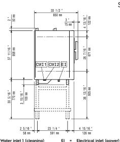
CWII Cold Water inlet 1 (cleaning) = Cold Water Inlet 2 (steam generator) CWI2
